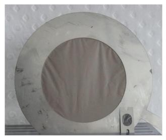
Figure 1: 80mm ultra-thin carbon foil for the ASACUSA experiment at CERN. On the bottom right a standard 90mm<sup>2</sup> frame as used at the MLL experiments is shown.
