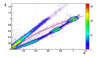
Figure 1: Slow decay constant factor  $(N_s)$  as a function of the fast decay constant factor  $(N_f)$  of CsI(Tl). The  $\gamma$ -rays (top curve) can be distinguished from the protons (bottom black curve). Punched-through protons can also be identified, as indicated by the red curve. Figure and details from [3]
