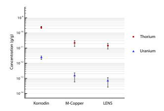
Figure 1: Concentrations of uranium and thorium in copper alloy (Korrodin), machine copper (M-Copper) and high purity copper (LENS) detected by AMS. [3]
