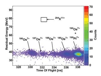
Figure 1: All events collected with settings on the superheavy isotope  $^{294}X^{11+}$  (arbitrary element X). Black box represents the region of interest at  $1\sigma$  around the calculated expected signal.
