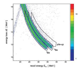
Figure 1. ERD measurement of <sup>9</sup>Be and <sup>10</sup>Be. Shown is the energy loss versus the total energy of both <sup>9</sup>Be and <sup>10</sup>Be. Indicated are the regions of interest as well as the region which we took for the pile up correction.
